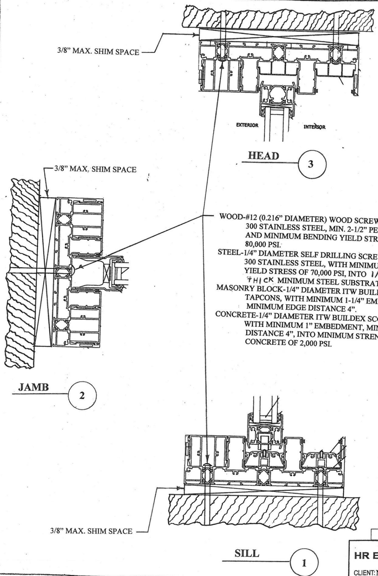
WOOD-#12 (0.216" DIAMETER) WOOD SCREWS, SERIES 300 STAINLESS STEEL, MIN. 2-1/2" PENETRATION, AND MINIMUM BENDING YIELD STRESS OF 80,000 PSI.
